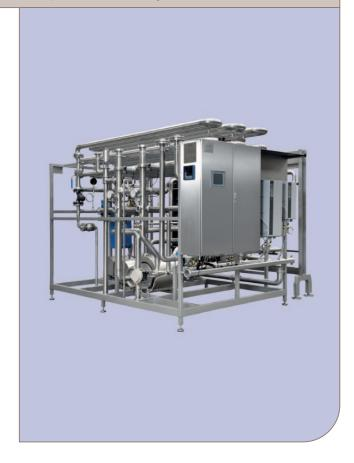
The incoming flow of cold yeast is heated to the target temperature for thermolyzation in two steps, using a high-efficiency Alfa Laval plate heat exchanger. The yeast is first heated in the heat recovery section, where it circulates against already thermolyzed yeast, and then in a heating section, in which circulating hot water is used to bring the yeast to the specified temperature.
